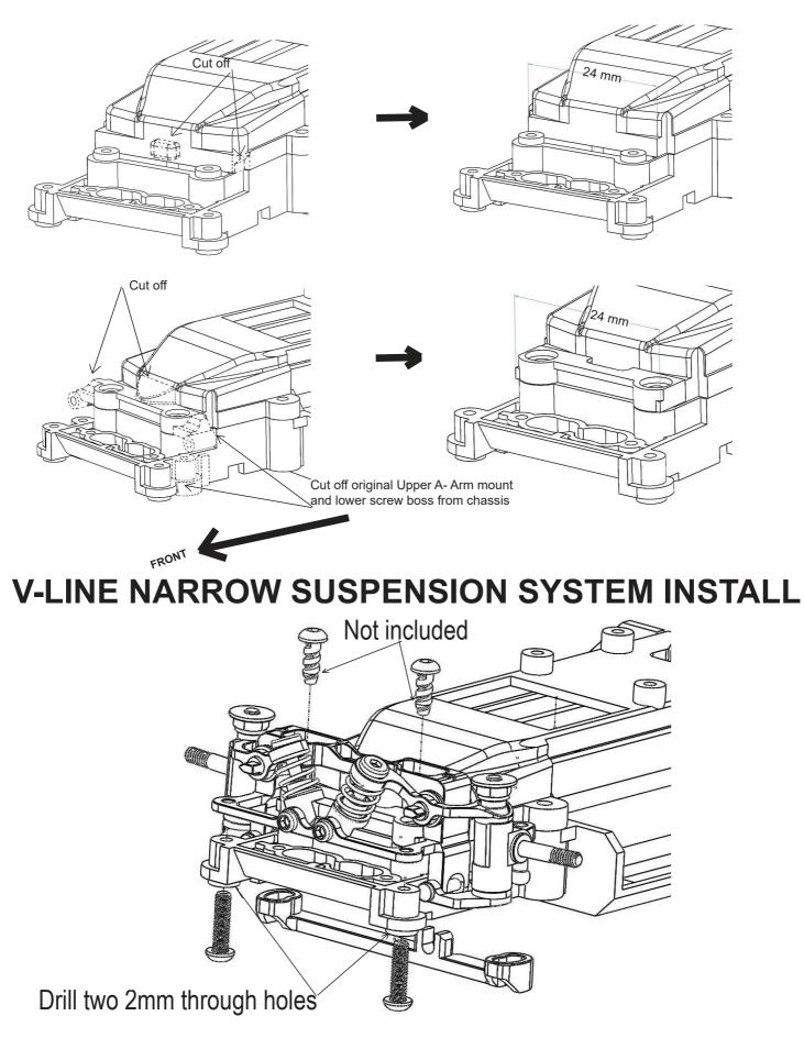
Slide the V-line Narrow Suspension system into original upper A-arm holes position then tighten 4 mounting screws to seat the V-line on chassis
