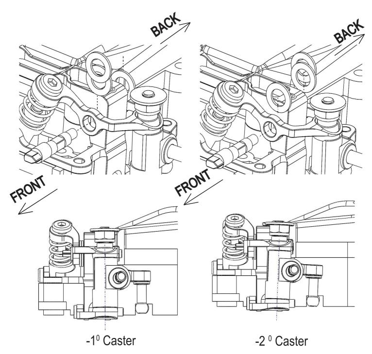
Loosen the Phillip screw then move cam shaft forward (FRONT) and fill two wahser in to the gap bettwen Upper Arm and Bracket (FRONT), one washer in to the gap bettwen Upper Arm and Braket (Back) have (-1 ° Caster) fill one wahser in to the gap bettwen Upper Arm and Bracket (FRONT), two washer in to the gap bettwen Upper Arm and Braket (Back) have (-2 ° Caster)
