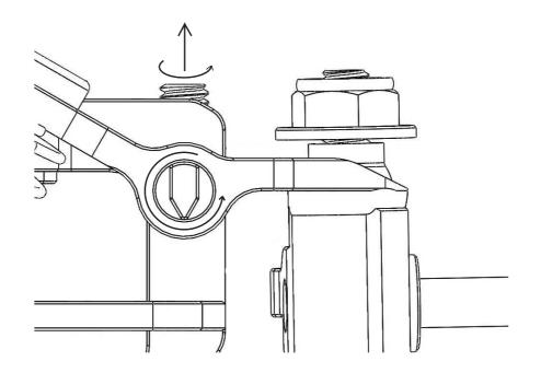
Loosen the flat point screw then rotate shaft 90° 180° 270° corresponding to the statics camper which you choose
